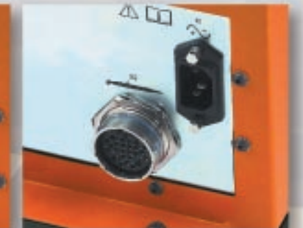
The standard TMEM is very simple – only 3 connectors – power, tool, and serial for programming.
