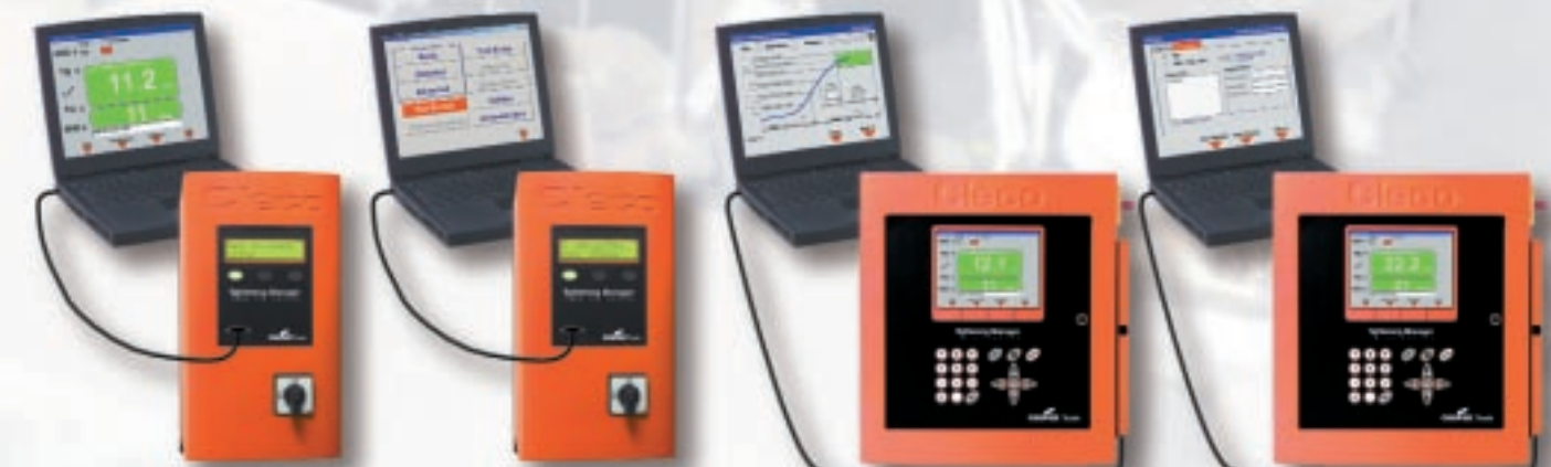
TM-COM1M connected to standard TMEM via RS232 serial.
